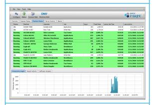
The top section shows a list of all machines at the site: Green indicates that the machine is running; no highlight indicates that the machine is idle. The bottom section provides a minute-by-minute graph of the selected machine's productivity.
