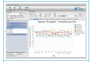
This report compares operator throughput (transactions per hour) on a month-by-month basis, across an entire year. The selected job (Applications) has a target rate of 850 transactions per hour, shown as the blue "Target" line.
